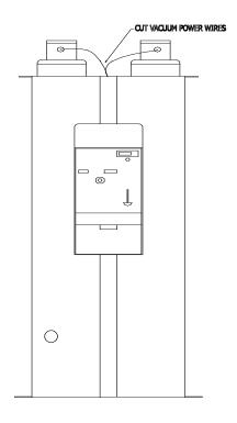
4. CONNECT THE TWO WIRES FROM THE VACUUM MOTORS (THE CUT WIRES) TO THE TWO HARNESS WIRES LABELED **TO VAC MOTORS**. (BLACK TO BLACK AND WHITE TO WHITE). THE ACTUAL WIRE COLORS MAY VARY DEPENDING ON MANUFACTURER. IF SO CONSULT THE VACUUM UNIT OWNERS MANUAL.
