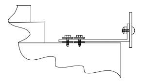
9. THE AIR SHAMMEE OUTER HOUSING SHOULD NOW BE SECURE TO THE TOP OF VACUUM. THE NEXT STEP IS TO WIRE THE UNIT TO THE VACUUM SYSTEM. THIS PROCESS IS COVERED IN THE NEXT SECTION. THE WIRING REQUIRES SOME WORK ON THE UNIT WITHOUT THE MOTOR PLATE INSTALLED, DO NOT INSTALL THE MOTOR ASSEMBLY AT THIS TIME!
